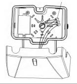
4. Tighten the screw to close the lamp.
