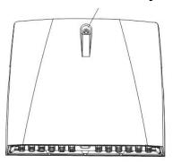
2. Use screws to install the lamp onto the solid wall.
