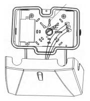
3. Connect the input wire, and then tighten the connector.
